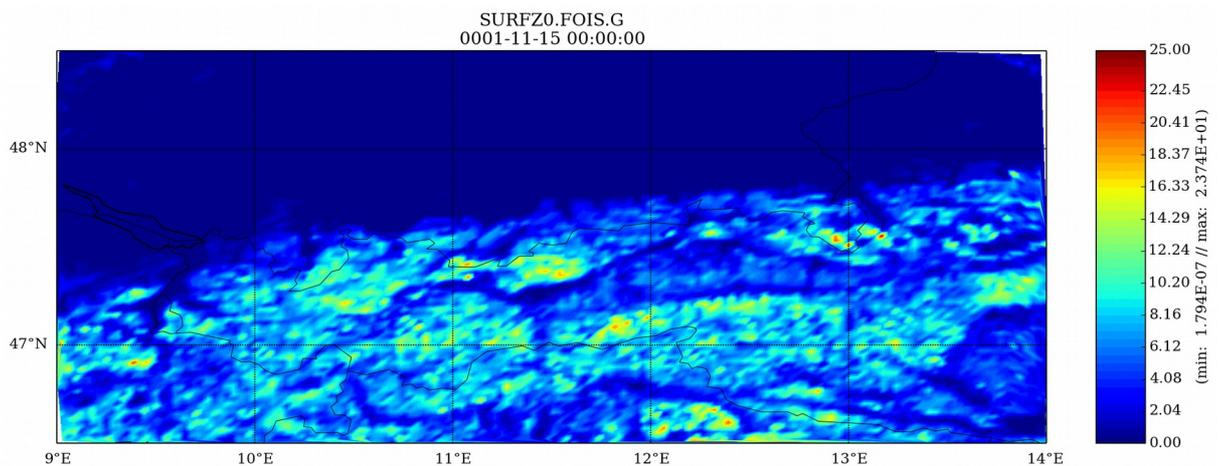
Figure 2.4: MOD\_923 Roughness length  $Z_0$  [m] (divided by  $g$ ) in 2.5km atmospheric ISBA clim file after replacement with SFX.ZOREL from SURFEX output
