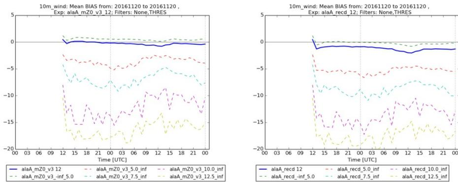
Figure 3.21 - 3.22.: 10m wind speed bias for different thresholds for ALARO 2.5km runs “alaA\_mz0\_v3” (left) and “alaA\_recd” (right) for the model run 20161120 12 UTC
