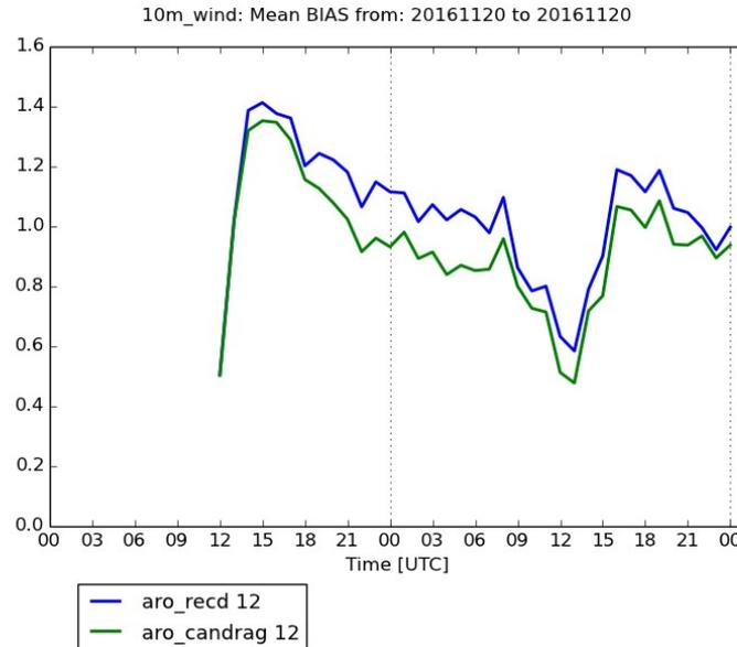
Figure 3.14.: 10m wind speed Bias based on all (roughly 250) automatic weather stations in Austria for the model run 20161120 12 UTC. Model shown: AROME “aro\_recd” and AROME with activated LCANOPY\_DRAG “aro\_recd\_candrag”.
