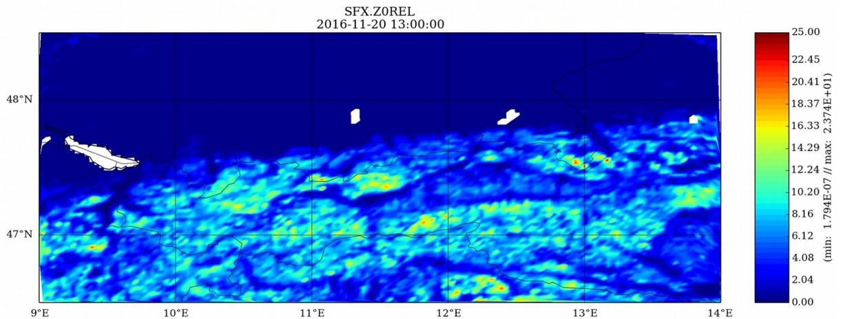
Figure 2.1 – 2.3: Roughness length  $Z_0$  [m] version “DEF\_923” as seen in ISBA climate file after conf 923 in SURFZO.FOIS.G (divided by  $g$ ) in the 4.8km (top) and 2.5km (middle) case. Bottom: “DEF\_PG D” roughness length (SFX.ZOREL) for 2.5km; zoom over western part of Austria (Vorarlberg, Tyrol and surroundings)
