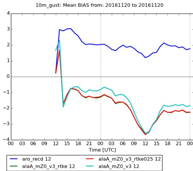
Figure 4.3.: Bias based on all Austrian weather stations (roughly 250) for different gust options in ALARO 2.5km and for AROME for the model run 20161120 12 UTC
