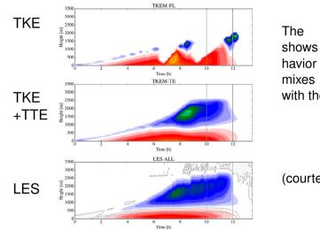
The two-energy scheme shows a more continuous behavior in time and space and mixes deeper in accordance with the LES results.
