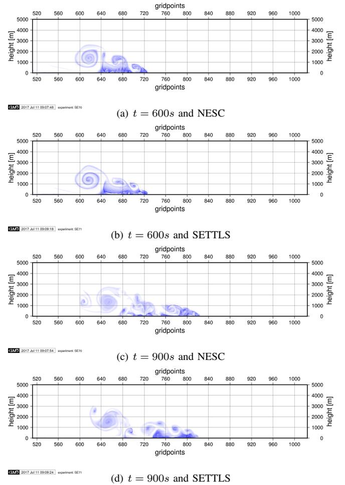
Figure 5: Density flow simulation after 600s and 900s. Simulations are performed with  $\Delta t = 3s$  and with no diffusion.
