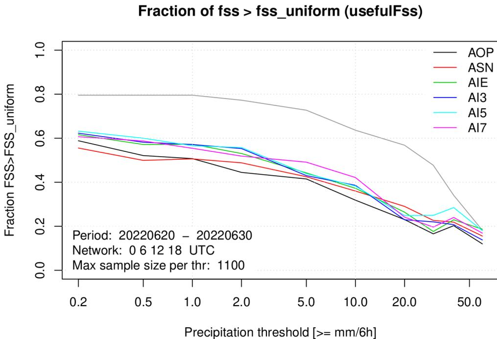
Figure 12: The fraction of forecasts which are useful ( $FSS > FSS_{uniform}$ ). The grey line shows the percentage of cases when both observed and forecasted precipitations exceed the defined threshold at least at one point.
