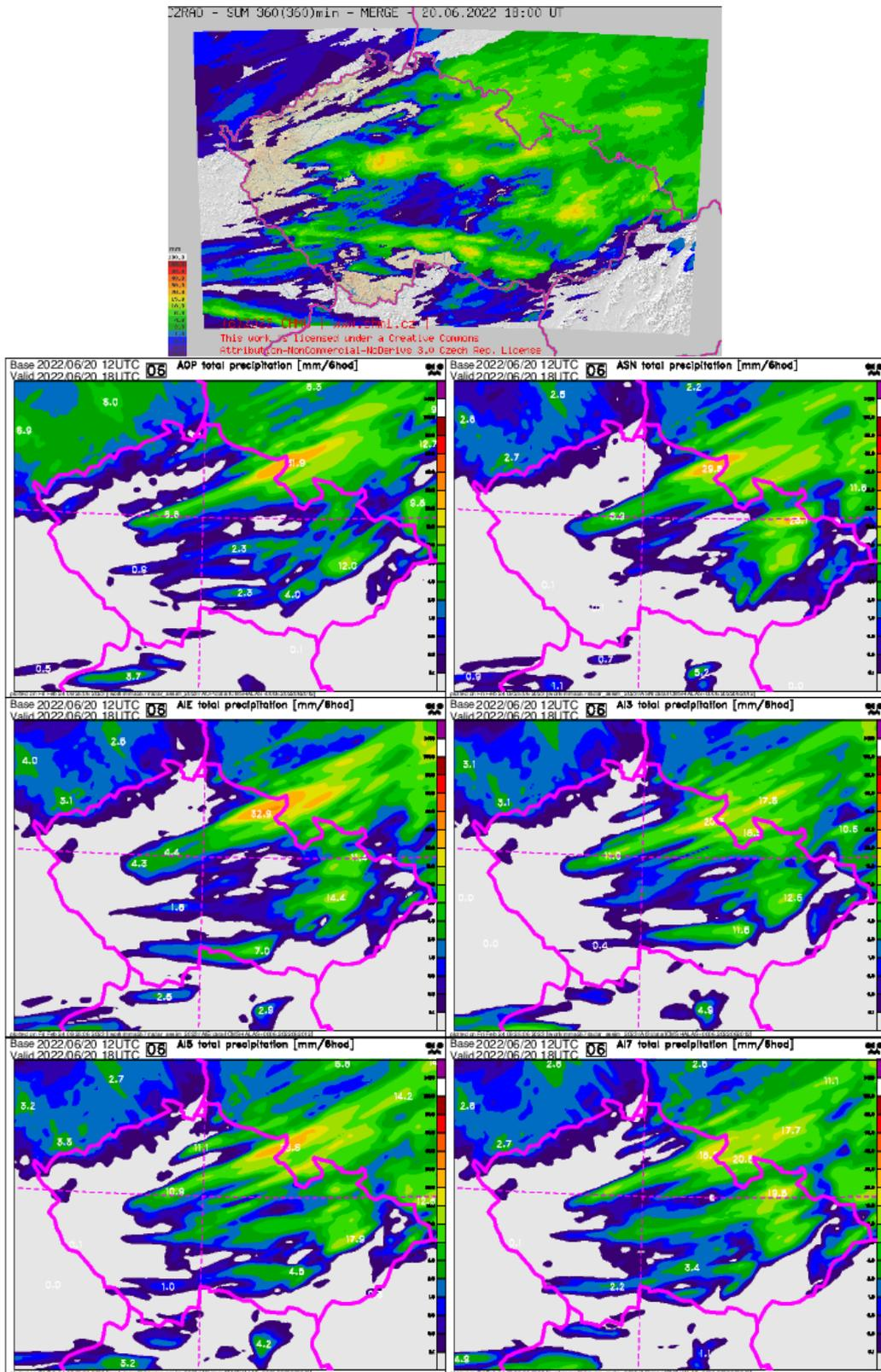
Figure 13: The 6h precipitation forecast for 20 June 2022 12UTC for lead time of +06h for experiments AOP, ASN, AIE, AI3, AI5 and AI7 and observations – radar and rain gauges based quantitative precipitation estimate (top).
