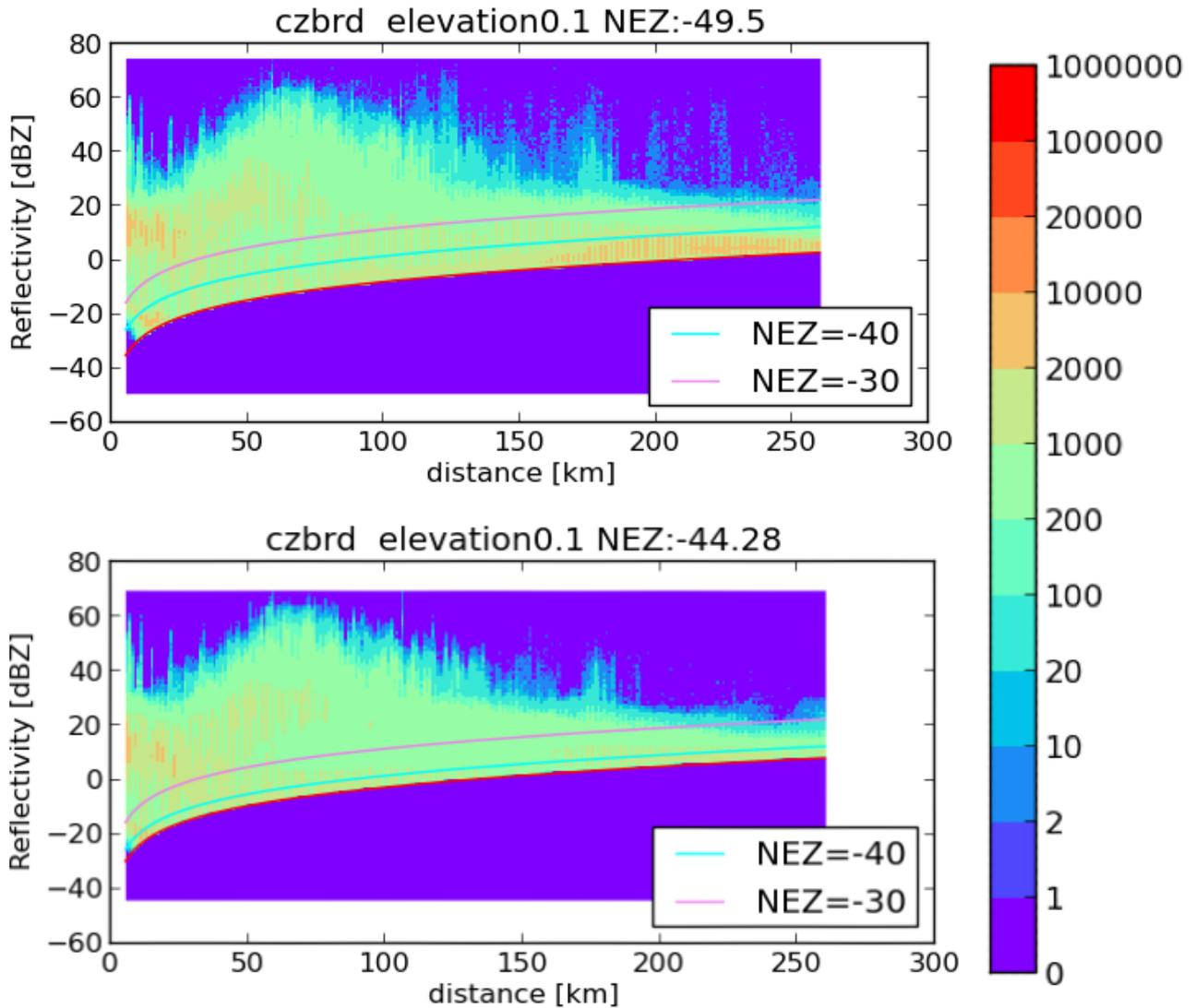
Figure 1: Radar czbrd 0.1 elevation TH data heatmap with calculated MDRF values (NEZ in OPERA files) for 09.01.2023 (upper picture; NEZ=-49.5) and 11.01.2023 (lower picture; NEZ=-44.28).
