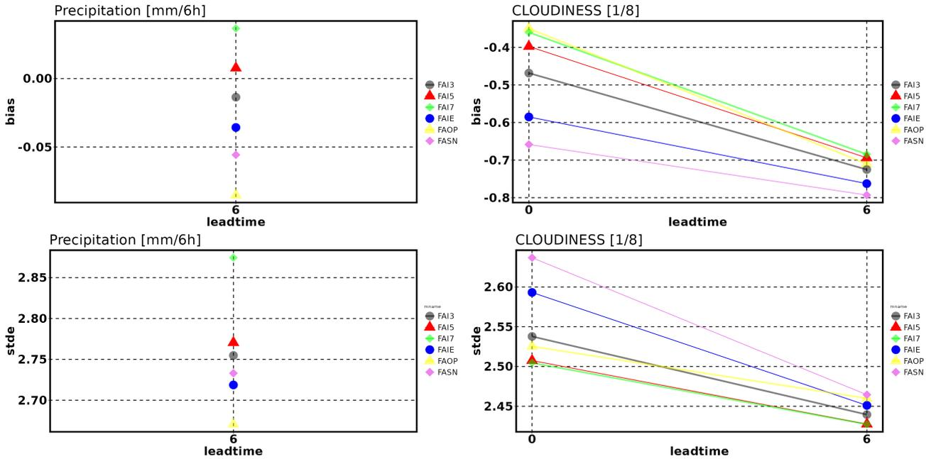
Figure 11: BIAS (upper pictures) and STDE (lower pictures) of the 6h precipitation accumulation and cloudiness for reference experiment AOP and radar experiments ASN, AIE, AI3, AI5, and AI7 over the assimilation period of 20-30 June 2022 for all network times (00, 06, 12 and 18 UTC).
