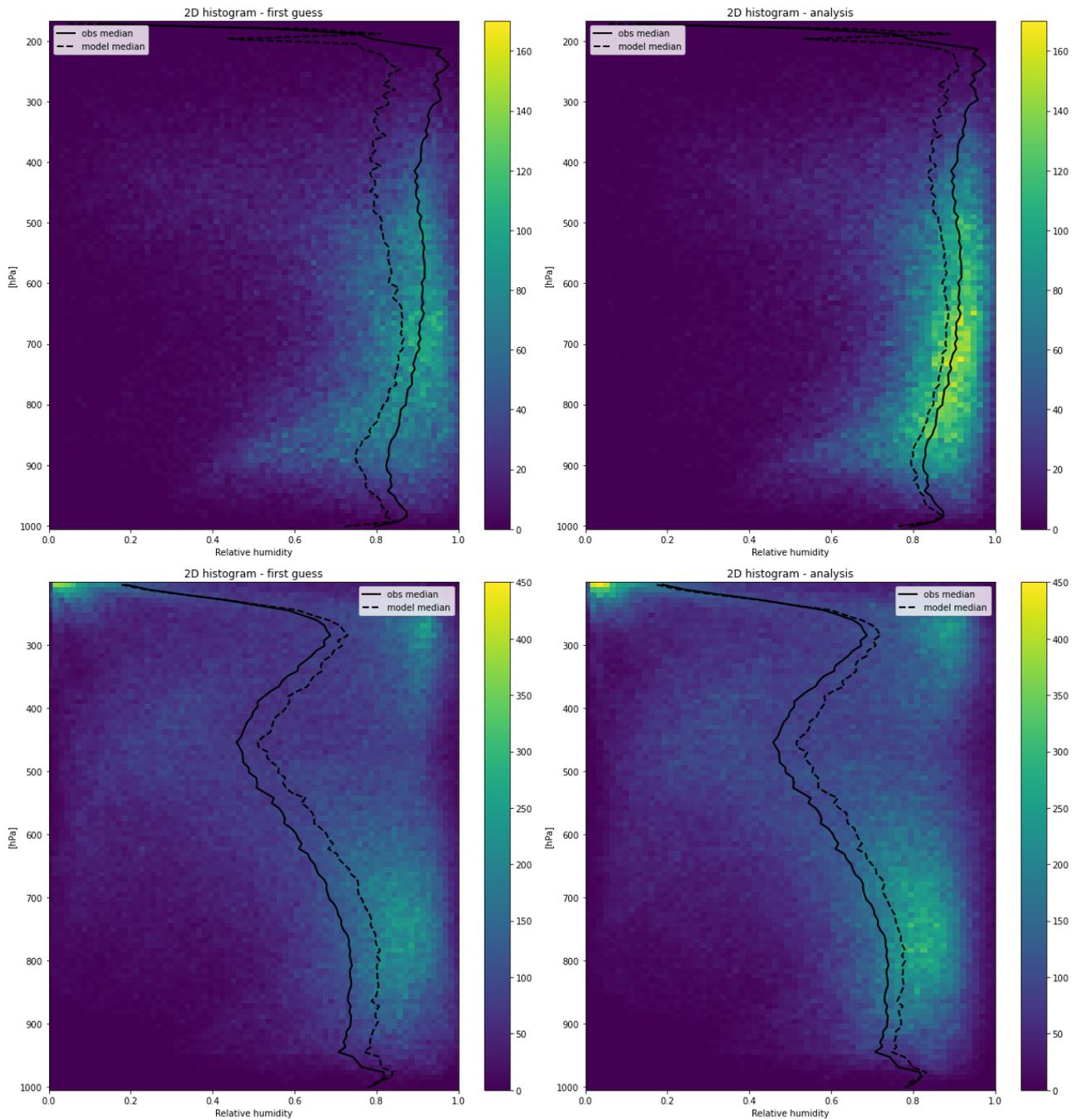
Figure 9: 2D histogram of RH model values at observation locations for a period of 20-30 June 2022. The relative humidity per height for AI3 experiment first guess (left pictures) and analysis (right pictures); split by type of observation: wet (upper pictures) and dry (lower pictures).
