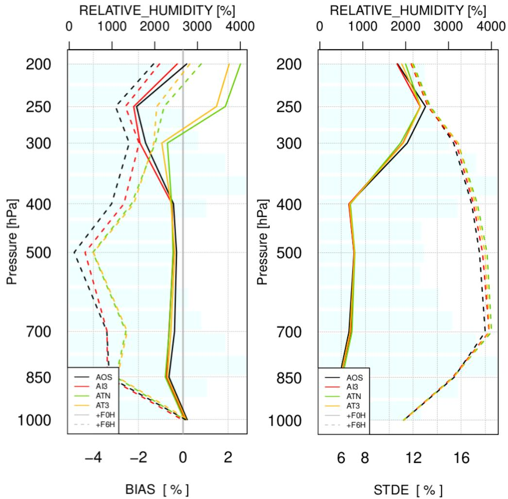
Figure 22: BIAS (left) and STDE (right) of relative humidity for reference experiment AOP and radar experiments ATN, AT3 and AI3 over the assimilation period of 8-18 January 2023 for all network times (00, 06, 12 and 18 UTC).
