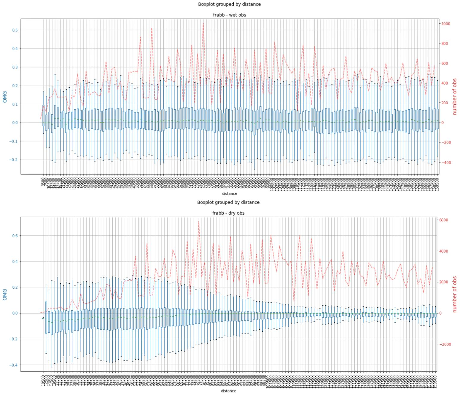
Figure 5: Radar frabb - boxplot of first guess departures grouped by distance from the radar (blue) and number of observations at the selected distance (red); split by type of radar observation data - wet (upper picture) and dry (lower picture).
