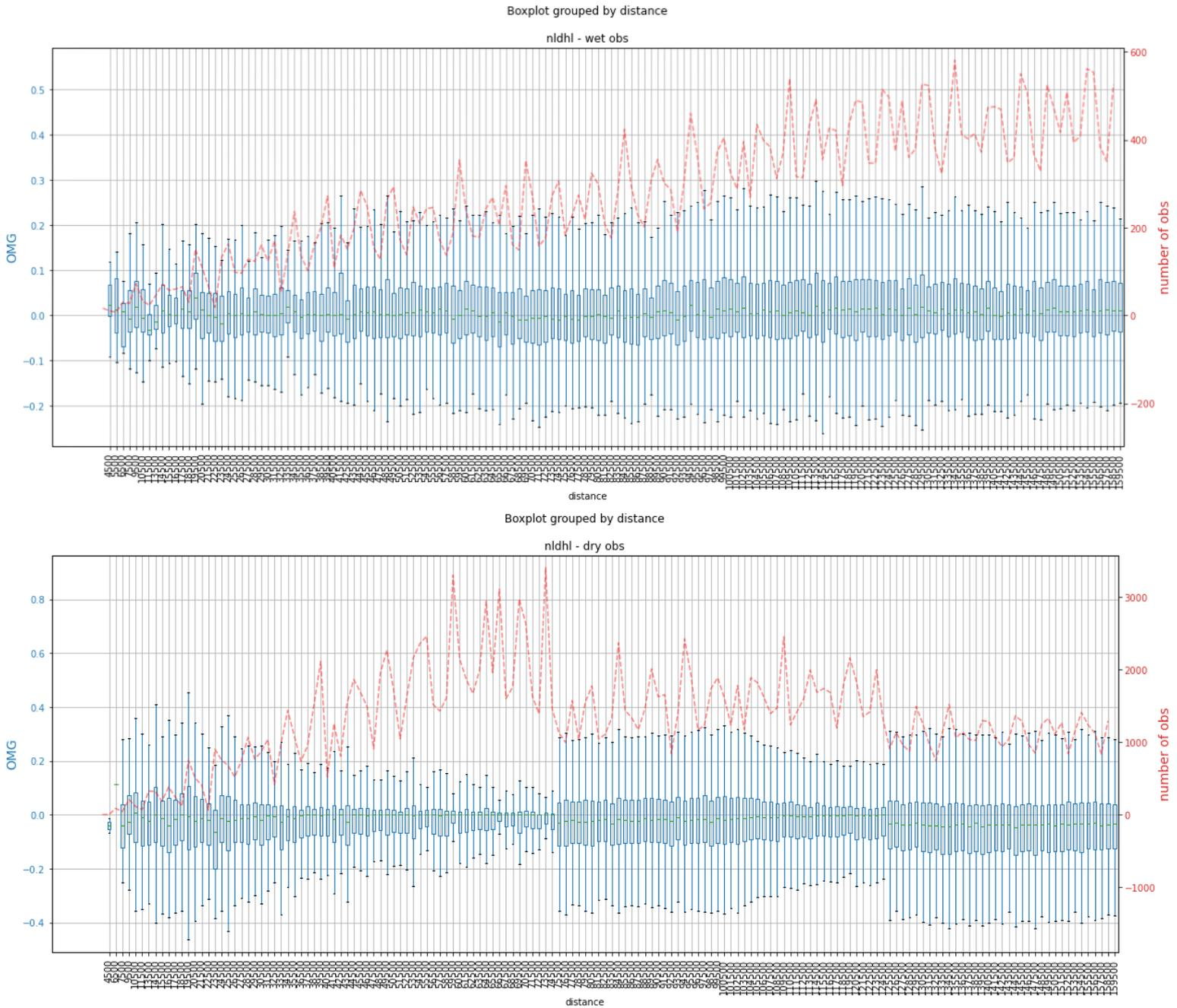
Figure 6: Radar ndhl - boxplot of first guess departures grouped by distance from the radar (blue) and number of observations at the selected distance (red); split by type of radar observation data - wet (upper picture) and dry (lower picture).
