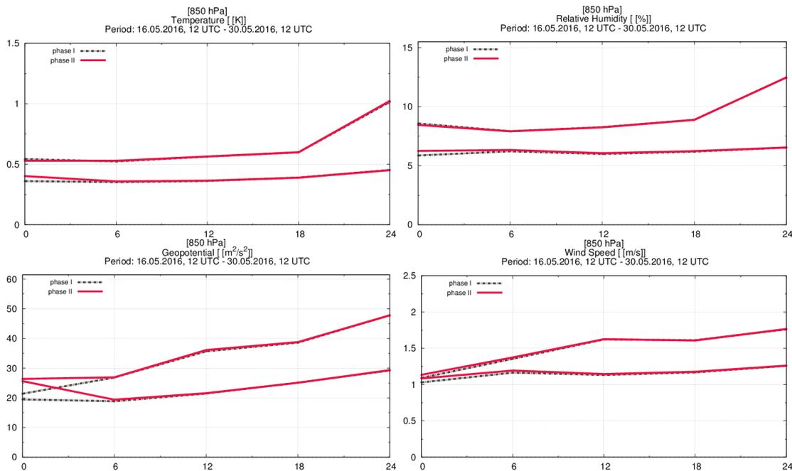
Figure 17: 850 hPa RMSE (upper line) and spread (bottom line), the 3DVar has neutral impact, but spread has been improved (increase) in all cases.
