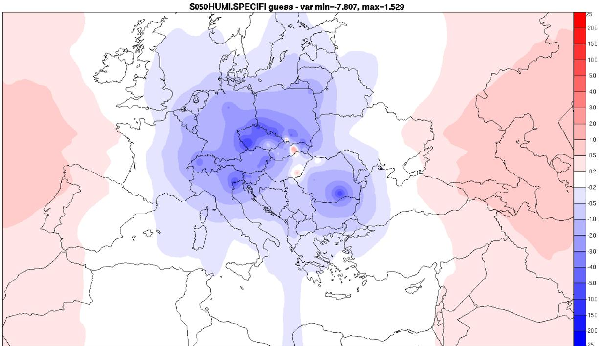
Figure 6: Increments in specific humidity [ $\text{g kg}^{-1}$ ] at model level 50 only from GNSS zenith total delay data assimilation.
