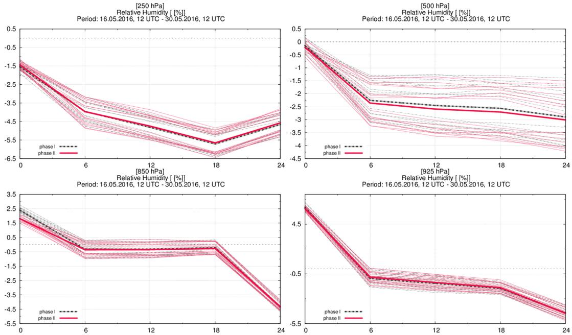
Figure 13: Relative humidity bias, small improvement was noticed in 850 hPa pressure level at time of analysis, but also small degradation at 6,12,18 and 24 hour forecast at 500 hPa level.
