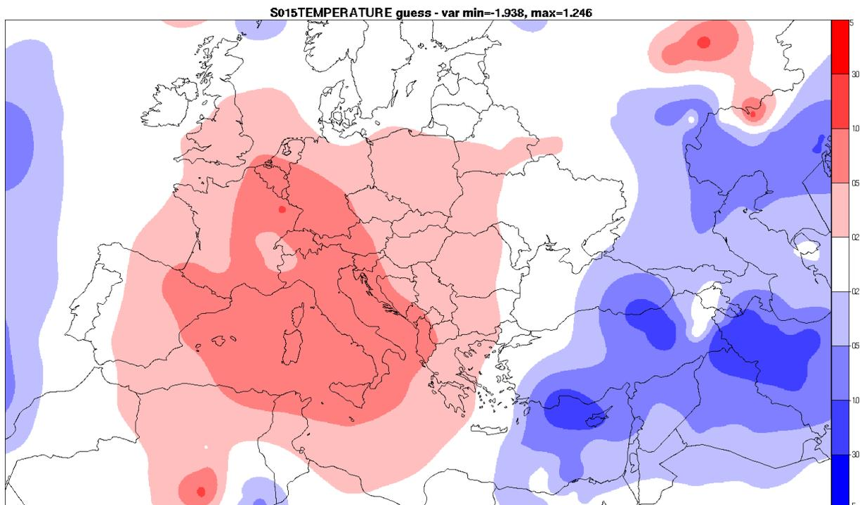
Figure 2: Increments in temperature [°C] at model level 15 only from AMDAR data assimilation.
