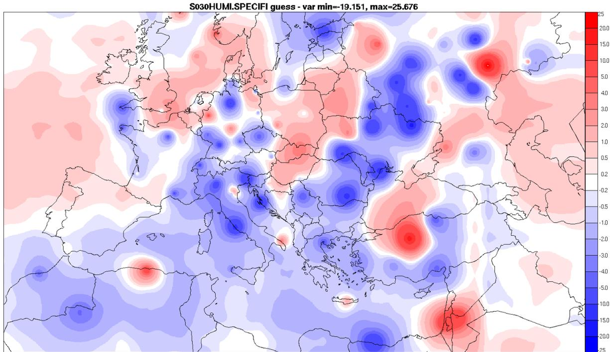
Figure 8: Increments in specific humidity [ $\text{g kg}^{-1}$ ] at model level 30 only from TEMP data assimilation.
