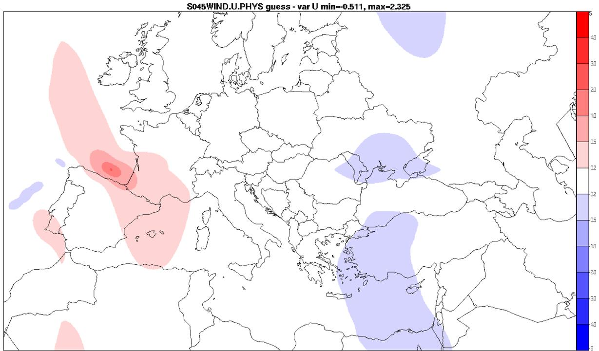
Figure 4: Increments in wind speed [ $\text{m s}^{-1}$ ] in direction U at model level 45 only from GEOWIND data assimilation.
