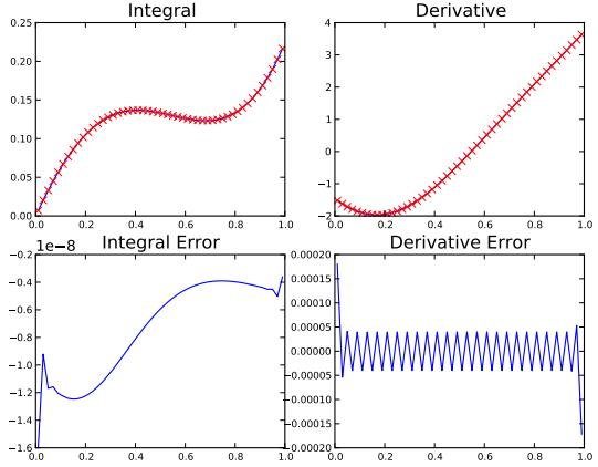
Figure 2: Derivative  $\mathbf{D}$  and integral  $\mathbf{Q}$  operators applied to the test function, for cubic B-spline and 50 full levels. Above, analytical values in blue, numerical values in red crosses. Below, the difference between numerical and analytical values
