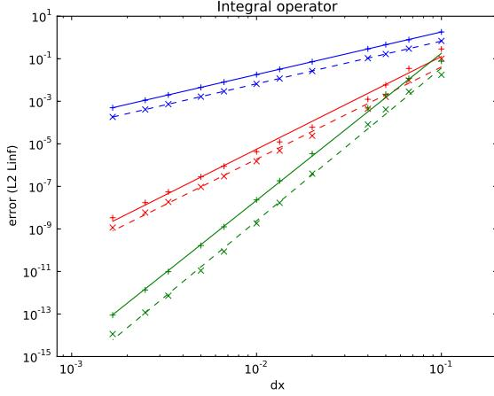
Figure 4: Convergence of integral operator  $\mathbf{Q}$ . Blue, red and green colors correspond to linear, cubic and quintic B-splines representation respectively. Continuous and dashed lines correspond to a linear logarithmic regression between the  $L_\infty$  and  $L_2$  errors and the grid spacing. The crosses are the errors when considering a number of levels equal to 10, 15, 20, 25, 50, 75, 100, 150, 200, 300, 400 and 600.
