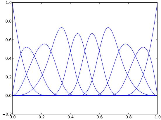
Figure 1: B-spline basis for  $N = 10$  full levels regularly spaced.
