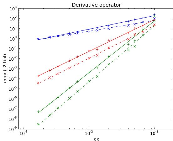
Figure 5: Convergence of integral operator  $\mathbf{D}$ . Blue, red and green colors correspond to linear, cubic and quintic B-splines representation respectively. Continuous and dashed lines correspond to a linear logarithmic regression between the  $L_\infty$  and  $L_2$  errors and the grid spacing. The crosses are the errors when considering a number of levels equal to 10, 15, 20, 25, 50, 75, 100, 150, 200, 300, 400 and 600.
