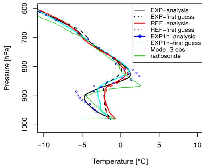
Figure 3. Slovenian case study comparing 3h RUC (black solid line) and 1h RUC (cyan solid line) temperature profile analyses. Mode-S observations (as reference) are signed by blue dots.
