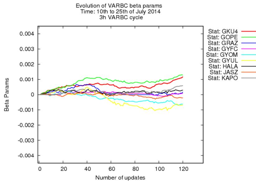
Figure 9. The 3 hourly VARBC cycling for GNSS ZTD observations. The evolution of VARBC  $\beta$  parameters for 9 different GNSS ground-based receiver stations.
