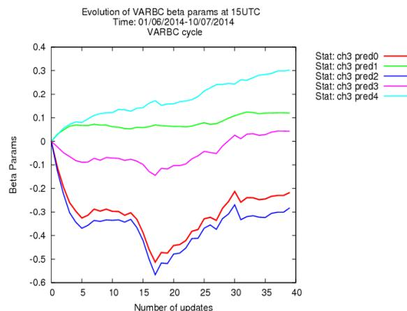
Figure 6. The evolution of  $\beta$  parameters for different predictors of VARBC for SEVIRI channel no 3 cycled at 15UTC analyses.
