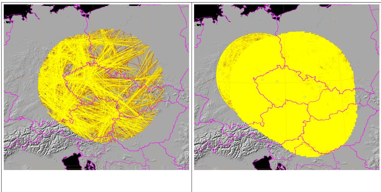
*Figure 10. The coverage of Czech Mode-S radars, 3 radars provides EHS and MRAR reports (on the left) and 5 radars provides only EHS (on the right)*
