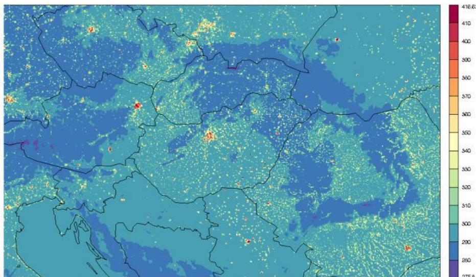
*Figure 4. 2m temperature at the end of assimilation window. Unrealistic high temperature can be seen over town tiles.*
