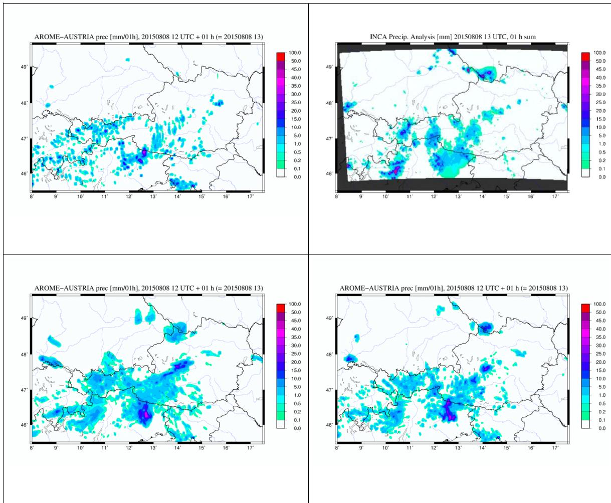
Figure 2. AROME/Austria precipitation case study comparing operational (upper left fig), INCA analysis (upper right fig), AROME with RADAR nudging settings no 1 (bottom left fig) and AROME with RADAR nudging settings no 2 (bottom right fig).
