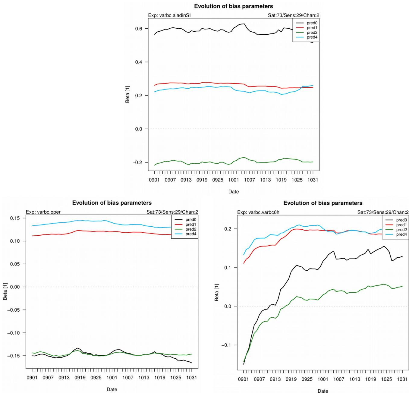
Figure 1: Evolution of VarBC coefficients for SEVIRI Ch.2 at 12 UTC in operational ALADIN/SI (top), ALADIN/CZ (bottom left) and experiment with 6-hour ALADIN/SI using only SEVIRI (bottom right).
