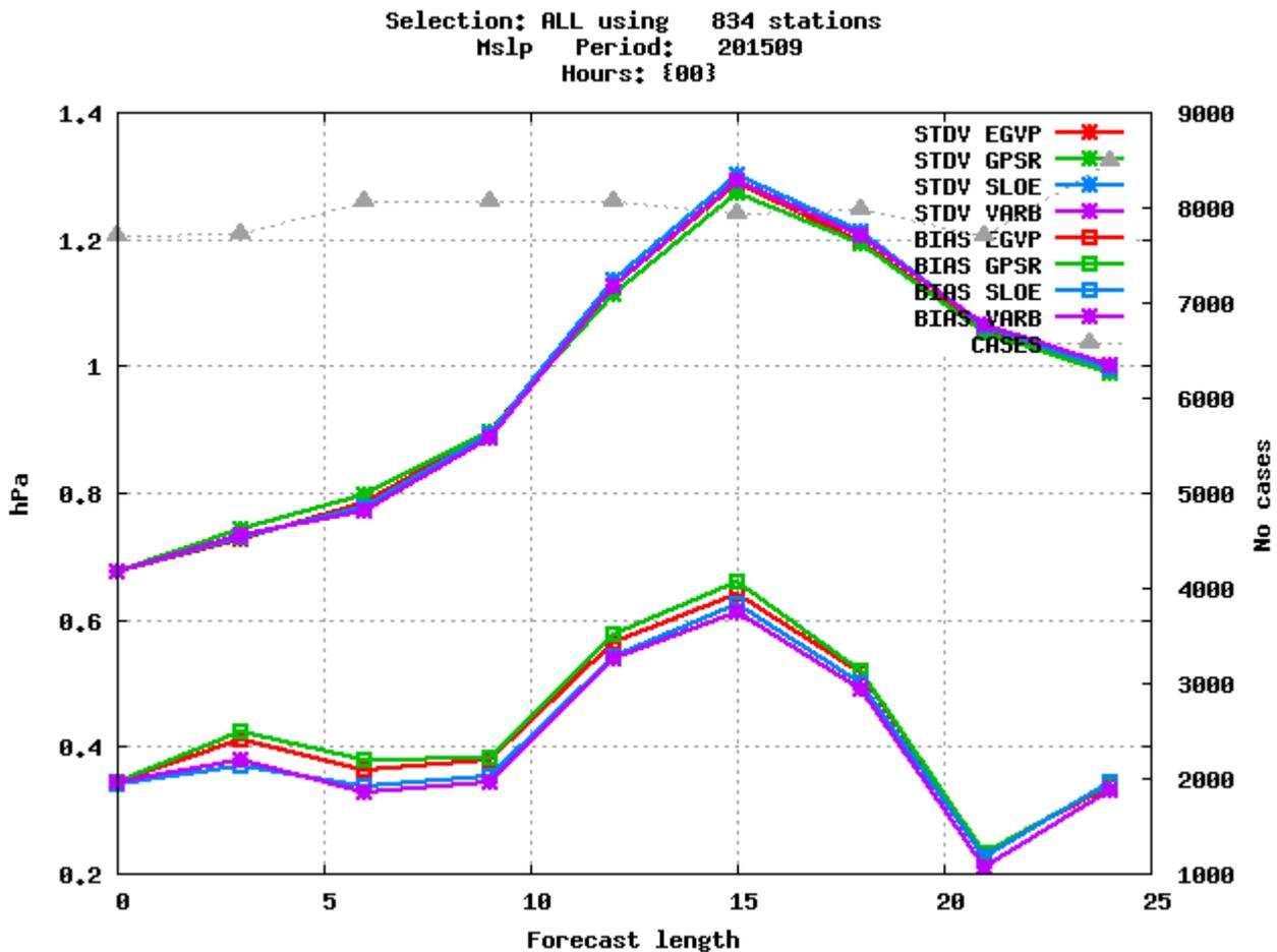
Figure 2: Verification of several GPS ZTD impact experiments against reference (green) for surface pressure over the operational domain for all network times
