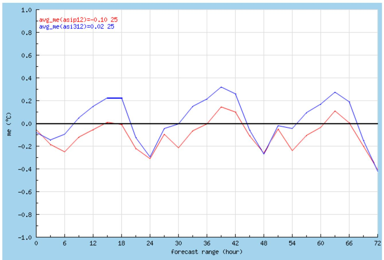
Figure 6: Bias of temperature at 2 m in operational reference (red) and LandSAF experiment (blue).
