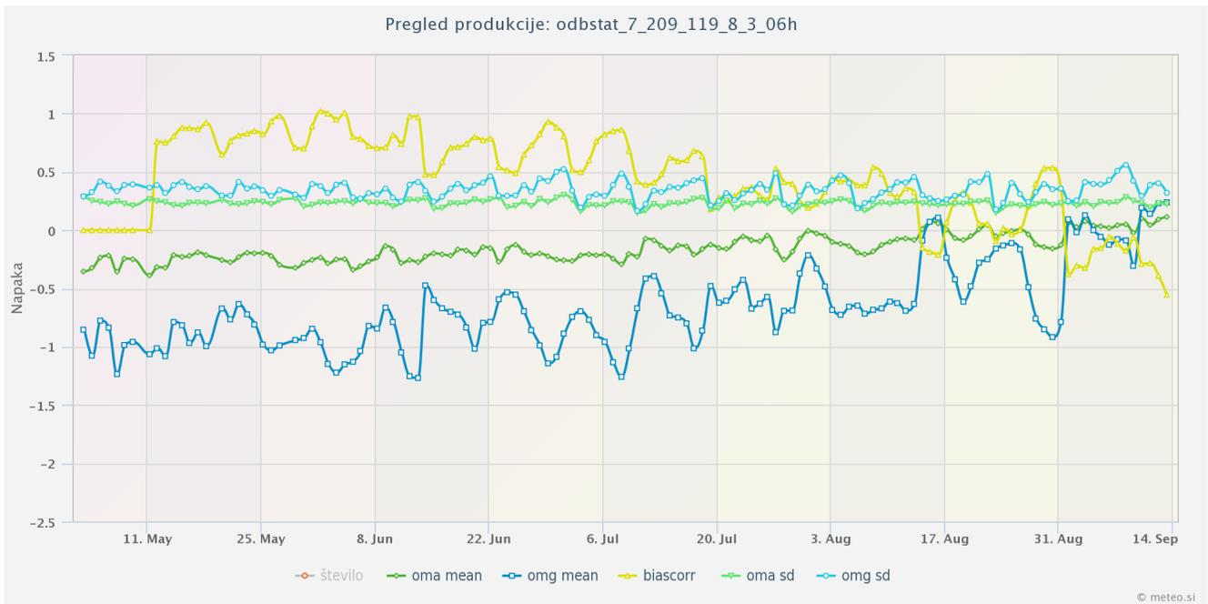
Figure 2: Time evolution of OMG and OMA mean and standard deviation, and correction as determined by Var-BC for SEVIRI ch.2 radiances at 3 UTC.
