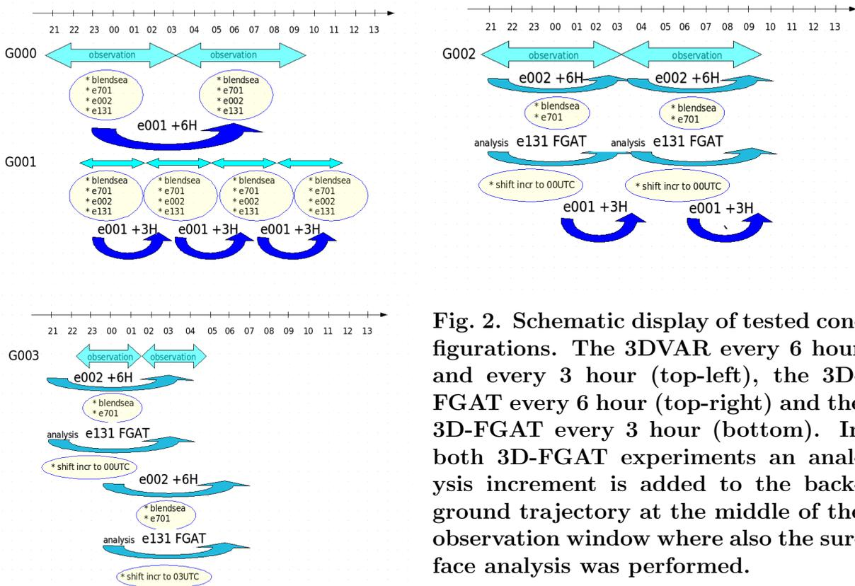
Fig. 2. Schematic display of tested configurations. The 3DVAR every 6 hour and every 3 hour (top-left), the 3D-FGAT every 6 hour (top-right) and the 3D-FGAT every 3 hour (bottom). In both 3D-FGAT experiments an analysis increment is added to the background trajectory at the middle of the observation window where also the surface analysis was performed.
