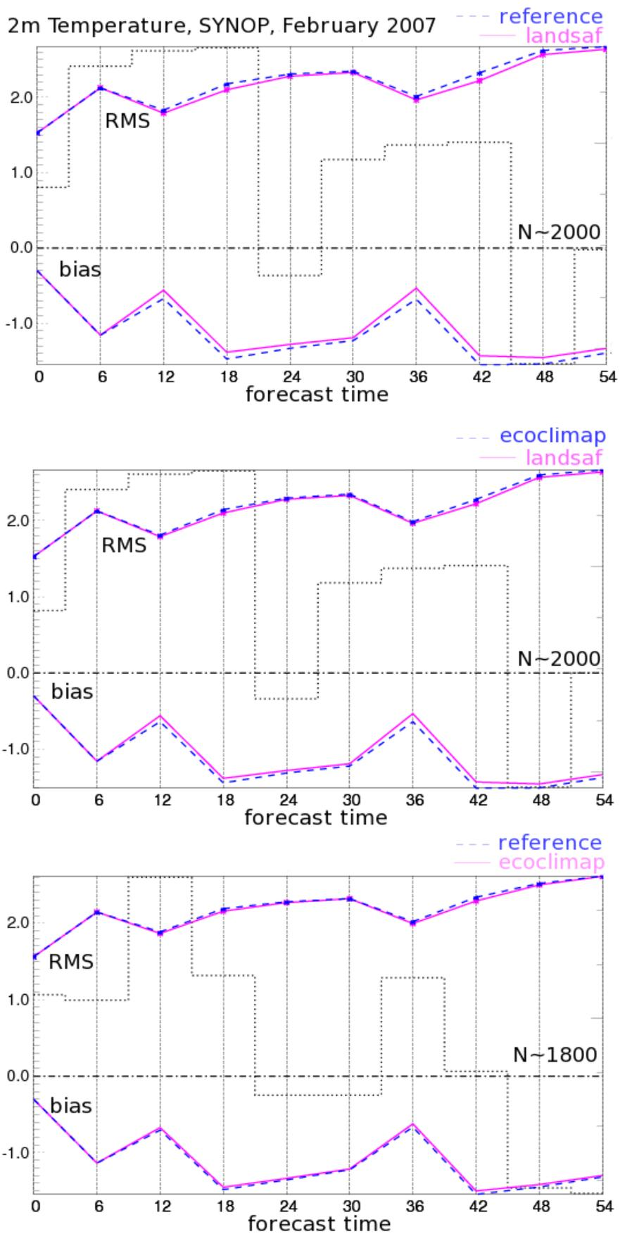
**Figure 3:** Statistical scores (bias and RMSE) for 2m SYNOP temperature for February 2007 for three pairs of experiments: a run with analyzed albedo (“landsaf”) compared to ALADIN “reference” (top), analyzed albedo run (“landsaf”) compared to ALADIN with albedo values from ecoclimap (“ecoclimap”) (middle) and ALADIN with ecoclimap (“ecoclimap”) values of albedo compared to a “reference” ALADIN run (bottom).
