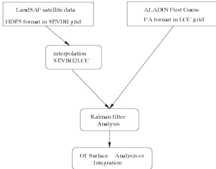
**Figure 1:** Dataflow of the redesigned experiment: the oval boxes are simple (one task only) programs and the process is controlled by a script. Such a design is quite suitable for a potential use in operational environment.
