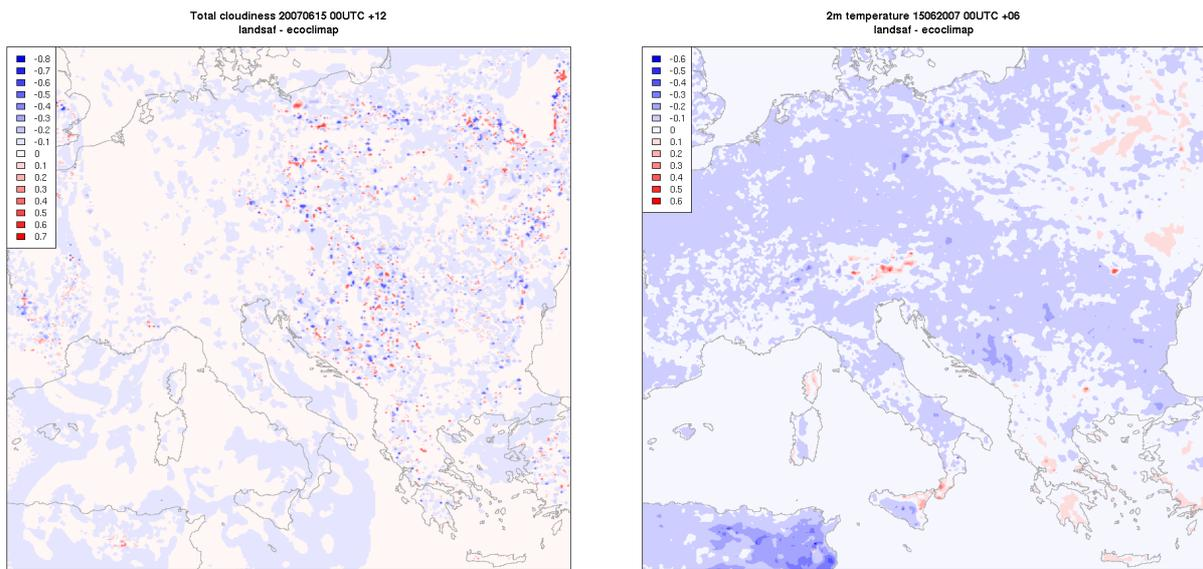
**Figure 6:** The difference in total cloud cover at noon (+12 hrs) (left) and early morning 2m temperature (at +6 hrs) for an early summer day (15<sup>th</sup> of June 2007) for the run with analyzed albedoes (“landsaf”) and the run with ecoclimap (“ecoclimap”) value of albedo.
