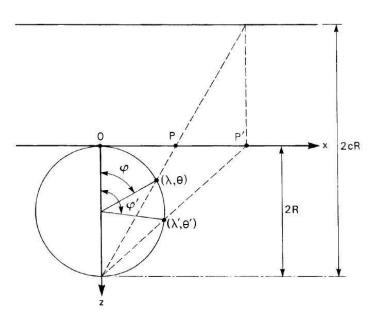
Figure 3: The transformation associated with a magnification in the complex plane (from Courtier and Geleyn)
