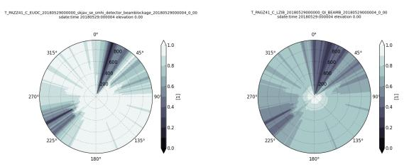
Figure 2: Beam blockage: OPERA (left) and QRAD (right) for skkoj (Kojsovska hola).
