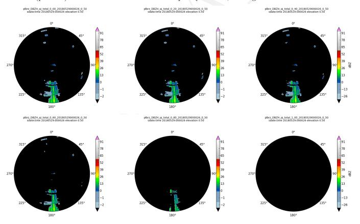
Figure 6: Filtered DBZH values below the threshold of 0, 0.2, 0.4 (top) and 0.6, 0.8 and 1 (bottom) of the OPERA total quality index (pl\_total) for plbrz (Brzuchania).
