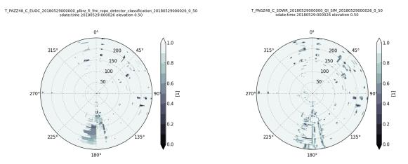
Figure 5: Non-met echo filter: OPERA (left) and QRAD QLSIM (right) for plbrz (Brzuchania).
