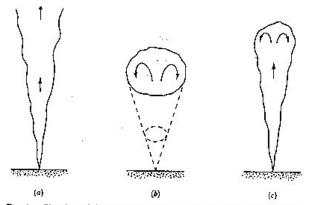
Fig. 6.1. Sketches of the various convection phenomena described in this chapter: (a) plume, (b) thermal, (c) starting plume. The arrows indicate the direction of mean motion, (From Turner 1969a.)
