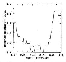
FIG. 13. The average downdraft measured in the 20 HIPLEX-1 clouds, as a function of the normalized distance from the upshear side of the cloud. The distance was normalized by dividing by the total length of the cloud penetration.
