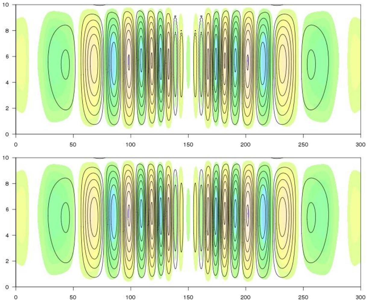
Figure 1: Potential temperature field in Baldauf-Brdar test (gravity waves in a channel); shading shows analytical solution, while contours represent solution with VFE (top) and VFD (bottom).
