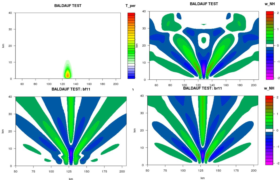
Figure 4: *Potential temperature perturbation in the lower atmosphere according to Simarro. Top left: initial field of potential temperature; top right: vertical velocity field after 600s – analytical solution; bottom: numerical solutions for VFE (left) and VFD (right).*
