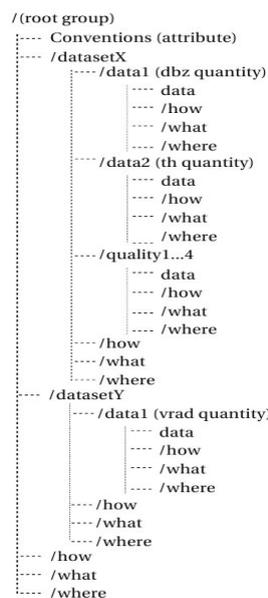
Fig.1 – Predetermined structure of the output HDF5 data file (Smerkol, 2018)
